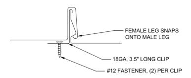
METHOD A: 24" O.C. METHOD B: 12" O.C. METHOD C: 6" O.C.
